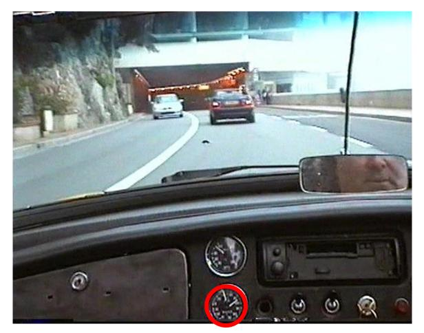
Don't be afraid of the temperature needle touching 212°F / 100°C on the gauge while the car is stuck in traffic, this is perfectly acceptable in a healthy car, so long as you expect to be driving at 4<sup>th</sup> gear speeds soon, to be able to bring the engine temperature back down to the normal range.
