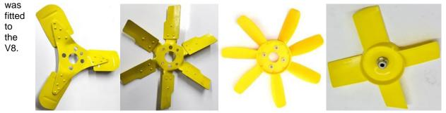
An electric fan is the only way to have enough air passing through the radiator of a performance tuned engine while the car is at a standstill for an extended length of time. A mechanical fan will spin at a lazy 700-850RPM when the MGB is at idle speed, which is nowhere near enough to draw sufficient air for a modified MGB engine that's stuck in traffic on a 40°C day. It's probably fine for a "sweltering" 26°C day at the height of an English summer.
